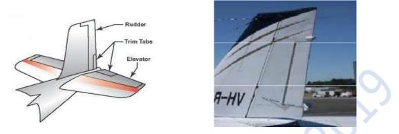
15. The rudder is a fundamental control surface, typically controlled bypedals rather than at the stick. It is the primary means of controlling yaw-the rotation of an airplane about its vertical axis. The rudder may also be called upon to counter-act the adverse yaw produced by the roll-control surfaces.
