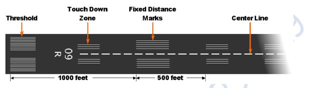
(b) <u>Runway Centre Line Markings</u>. Runway centre line markings shall consist of a series of broken longitudinal lines along the runway centre line and extending along the whole length of the runway
