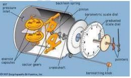
9. The whole assembly is encased in a container having an inlet for the static pressure but otherwise is airtight.
