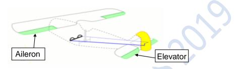
12. Ailerons are mounted on the trailing edge of each wing near the wingtips and move in opposite directions. When the pilot moves the stick left, or turns the wheel counter-clockwise, the left aileron goes up and the right aileron goes down. A raised aileron reduces lift on that wing and a lowered one increases lift, so moving the stick left causes the left wing to drop and the right wing to rise. This causes the aircraft to roll to the left and begin to turn to the left. Centering
