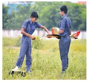
14. Power flight is not advisable till the gliding test is carried out successfully. For trial flight, a small amount of fuel is put into the fuel tank and the engine started by rotating the propeller. And the model launched gently the model should fly short distance and land perfectly.
