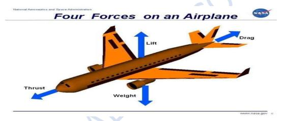
Lift and Drag are the most important components of aircraft in level flight. They act in 90<sup>0</sup> to each other. The Lift component of aircraft supports the aircraft in air whereas the drag resist the air craft movement in air.
