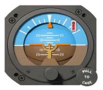
(a) The centre horizon bar separating the two halves of the display, with the top half usually blue in color to represent sky and the bottom half usually dark to represent earth.
