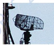
4. Radar is an object detection system which uses radio waves to determine the range, altitude, direction, or speed of objects. It can be used to detect aircraft, ships, spacecraft, guided missiles, motor vehicles, weather formations, and terrain. The radar dish or antenna transmits pulses of radio waves which bounce off any object in their path. The object returns a tiny part of the wave's energy to a dish or antenna which is usually located at the same site as the transmitter.
