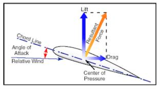
26. <u>Angle of Attack.</u> It is the angle between the chord line and the relative air flow undisturbed by the presence of aerofoil.
