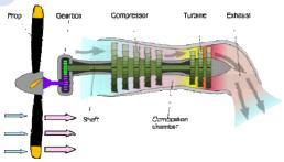
19. The main difference between single shaft and free turbine engine is in the transmission of power to the propeller.
