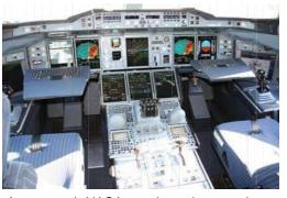
elements were competing for Cockpit space and pilot attention. As a result NASA conducted research on displays that could process the raw aircraft system and flight data into an integrated, easily understood picture of the flight situation, culminating in a series of flight demonstrating a full glass cockpit system.
